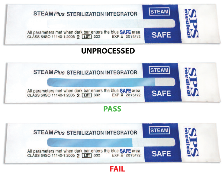
Figure 1. Class 5 integrators note whether a sterilization cycle has reached all three required parameters: time, temperature, and the presence of steam. They serve as an additional level of assurance in the sterilization process, and are used as an adjunct to the gold standard of biological monitoring.
